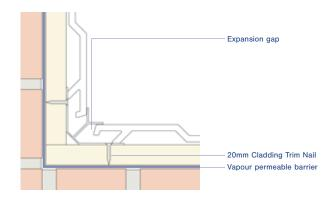
NB. Breather membrane is only required on non moisture resistant substrates
