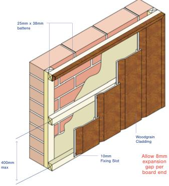
Working with Woodgrain cladding requires some modified procedures and installation processes. The following fixing details must be followed when installing Woodgrain cladding products:
